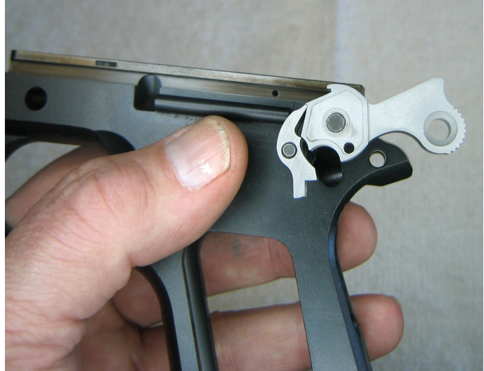
New Generation Lippard A3 Sear and Hammer illustrates the Anvil and Fulcrum release, allowing the opposing cam points to lift the A3 Hammer from the A3 Sear when firing.
