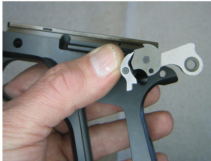
Conventional Sear and Hammer relationship illustrated with the patented Lippard A2 Sear and typical 1911A1 Hammer.
